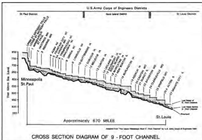
This graphic shows the lock & dam system on the Mississippi River. You can see the river bed as well as water depth both before and after the lock & dam system was built. The locks and dams maintain a nine foot channel which allows for shipping of goods on barges both up and down the river.
